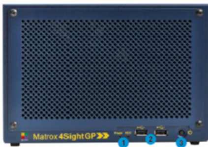
1. Status LEDs 2. USB 2.0 ports 3. Power switch
