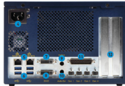
4. Power input 5. GbE ports 6. USB 3.0 ports 7. DVI-I output 8. DVI-D output 9. Audio in 10. Audio out 11. Auxiliary I/Os 12. PCIe slots
